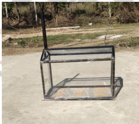
Fig. 3. Fabricated Chimney-assisted greenhouse solar dryer designs for wheat and paddy drying at the Department of Mechanical Engineering, AKS University, Satna (Madhya Pradesh), India.
